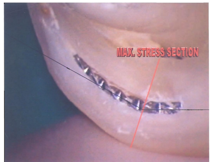
Fig. 18.17. In the rotary NiTi instrument working in a curved canal the tension and compression are at a maximum in correspondence to the cross section of the instrument where the radius of the curvature is the least.
